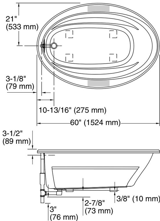
No change in measurements if connected with drain illustrated. (K-11677 or K-11677M)
