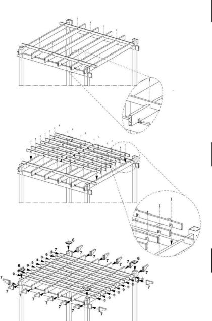
Using 2" painted screws, fasten top cross rails to upper supports.
