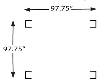
Using ground anchor installation layout drawing, dig holes 18" deep according to dimensions. Fill with cement and place ground anchors in wet cement. Be sure that ground anchors are straight and in accordance with dimension of ground anchor installation layout drawing. Allow cement to dry.
