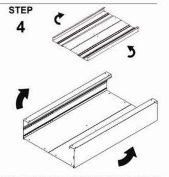
ROTATE FRONT EDGE OF BOTH SIDE PANELS UPWARD TO FORM RECTANGULAR CABINET SHAPE.
