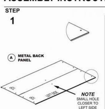
LAY METAL BACK PANELS ON FLOOR WITH INSIDE OF BACK PANEL FACING UP.
