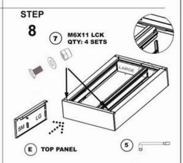
SLIDE TOP PANEL OVER THE SIDE, CENTER AND BACK PANELS. INSERT 4 - M6X11 BOLTS THROUGH FRONT AND FULLY TIGHTEN WASHER & LOCK NUTS FROM INSIDE USING M6 WRENCH.
