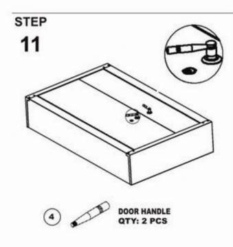
SCREW LOCK HANDLE INTO DOORS. OPEN AND CLOSE DOOR TO CONFIRM PROPER ALIGNMENT.
