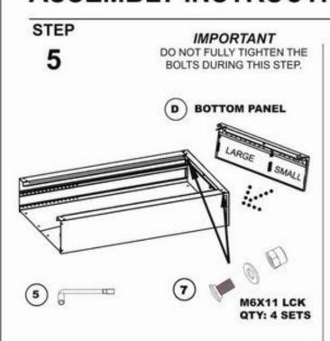
SLIDE BOTTOM PANEL OVER THE SIDE AND BACK PANELS. INSERT 4 - M6X11 BOLTS THROUGH FRONT AND LOOSELY TIGHTEN WASHER & LOCK NUTS FROM INSIDE.
