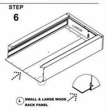
INSERT AND SLIDE 2 WOOD BACK PANELS INTO PLACE FROM TOP END OF CABINET.
