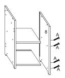
Use A screw to lock No.8 panel on No.2 and No.3 panel.
