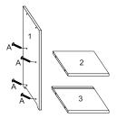
Use A screw to lock No.2 and No.3 panel on No.1 panel.
