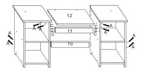
Insert C( wooden dowel) in No.11, use A screw to lock No.10 and 12 panel, joint to left and right parts.
