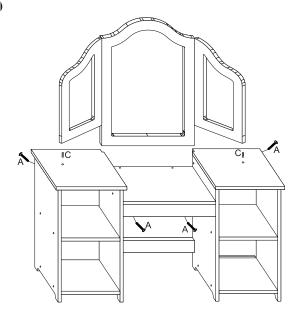
Insert C (wooden dowel) in No.14 and No.15, use A screw to lock it on table.
