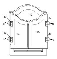
Use B screw to lock D(hinges) on No.13 ,No.14 and No.15 panel.
