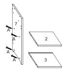
Use A screw to lock No.2 and No.3 panel on No.7 panel.
