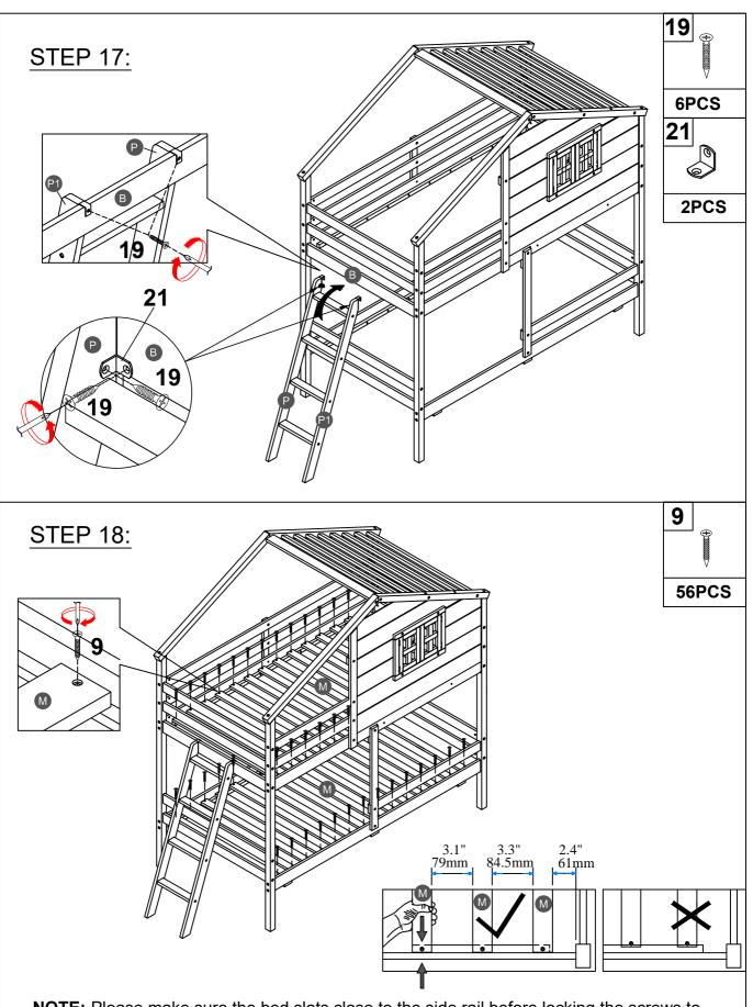
**NOTE:** Please make sure the bed slats close to the side rail before locking the screws to avoid breakage. This step is required for both the left and right sides. Moreover, please do not lock the screws of the bed slats at the outermost edge to avoid damaging.
