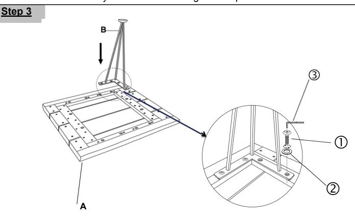
Insert leg (B) into the table top (A), put the flat washer (2) and bolt (1) as above picture.
