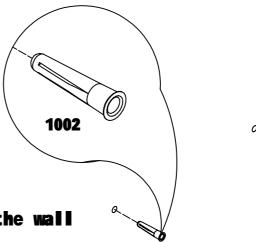
Make 10mm expansion holes on the wall
