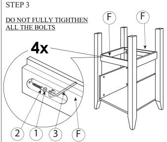
Turn the assembled leg part upright position, and assemble Rail (F) to the both leg frames (C) & (B).
