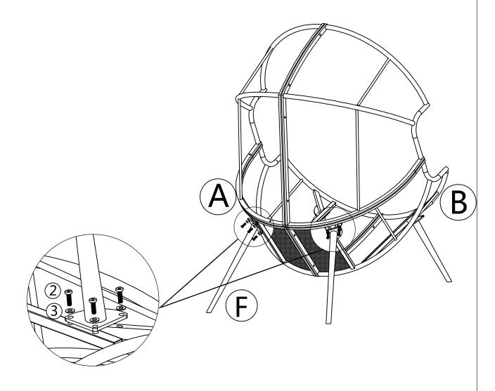
Adjust alignments and NOW TIGNTEN ALL SCREWS with wrench (5) with Allen key (6).
