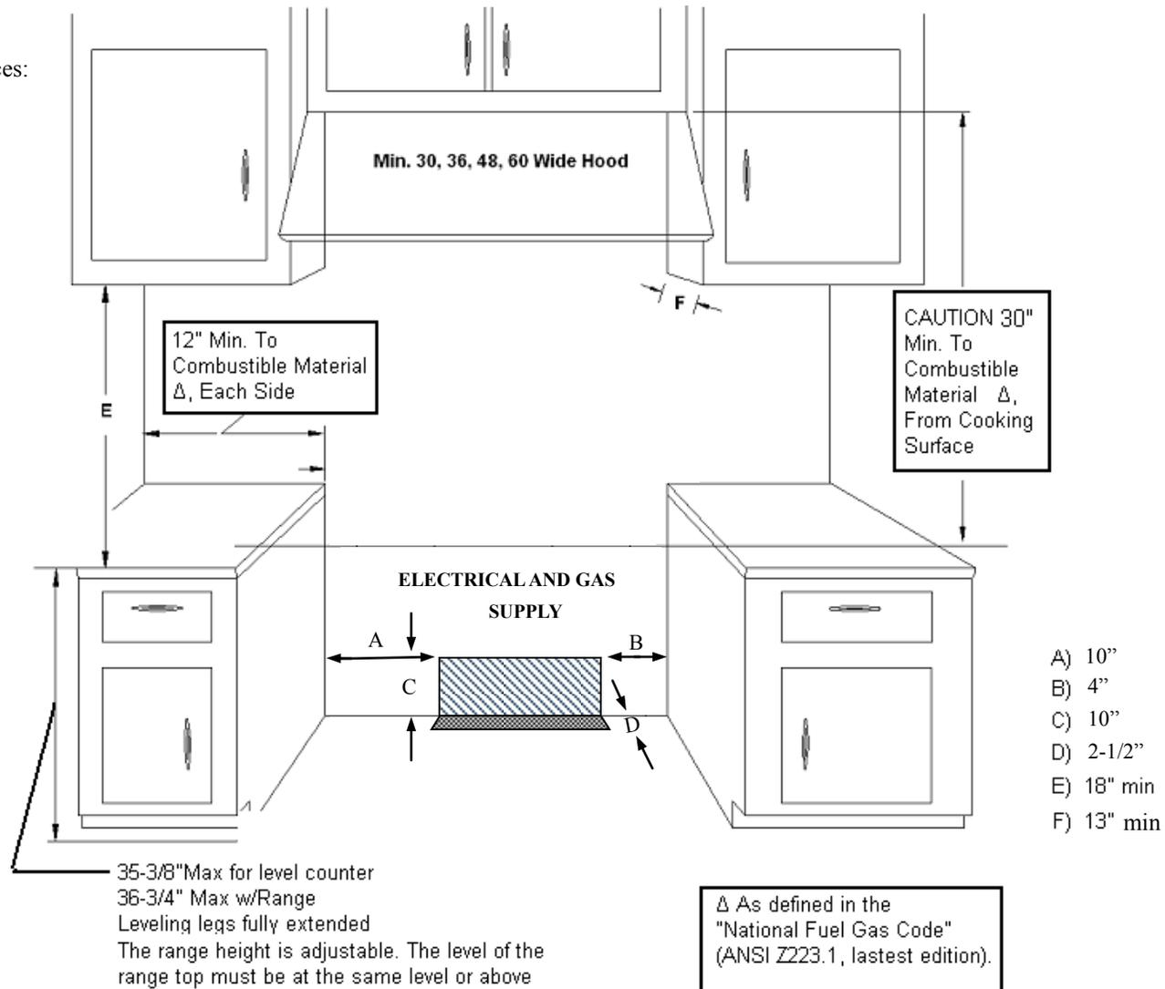
Range Widths    Cut Out Widths
