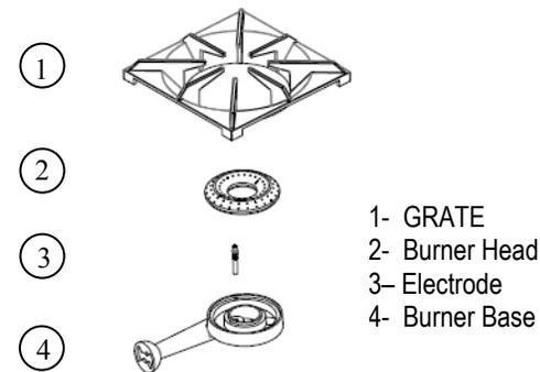
the grates and burners are cool, remove the grate. The Burner Cap can easily be removed. Wash these parts in hot soapy water, rinse and dry thoroughly. The Burner Caps are porcelain enamel, follow the directions on the previous page that were given for the burner grates. A bristle brush can be used to clean out the toothed burner ports, if necessary.
