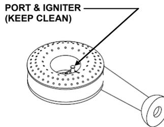
All the range-top burners have electronic spark ignition.
