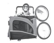
Step 1 Turn the still folded trailer around. Turn over the towing bar to be forward insert the safety lock to fix it.
