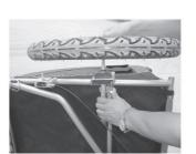
WARNING Both safety pins must be locked in place before using frailer. otherwise roll bar or tongue could shift and cause an accident or serious
