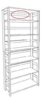
**STEP 2a**: Attach the Strap(**C**) to the highest cross brace that spans the back of your bookcase with 2 Small Screws(**A**).
