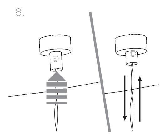
Pendant Cable length may be adjusted up and down by pressing in wire toggle and *gently* pushing /pulling cable
