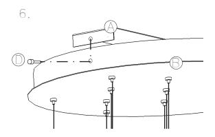
Remove chains from one side only, and attach  $\bigcirc$  to  $\bigcirc$  with the button head screws  $\bigcirc$
