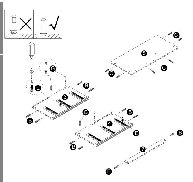
• The provided glue(G) is to secure wood dowels(A) in place. When first inserting dowels, locate the appropriate hole for the dowel, place a small amount of glue in the hole and insert the dowel. Wipe away excess glue immediately.
