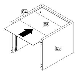
Step 4: Attach bottom panel (2) to side panel (3) and (4) using hardware C and D.
