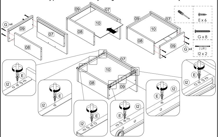
Step 8: Assemble the drawer in place along the drawer slides.
