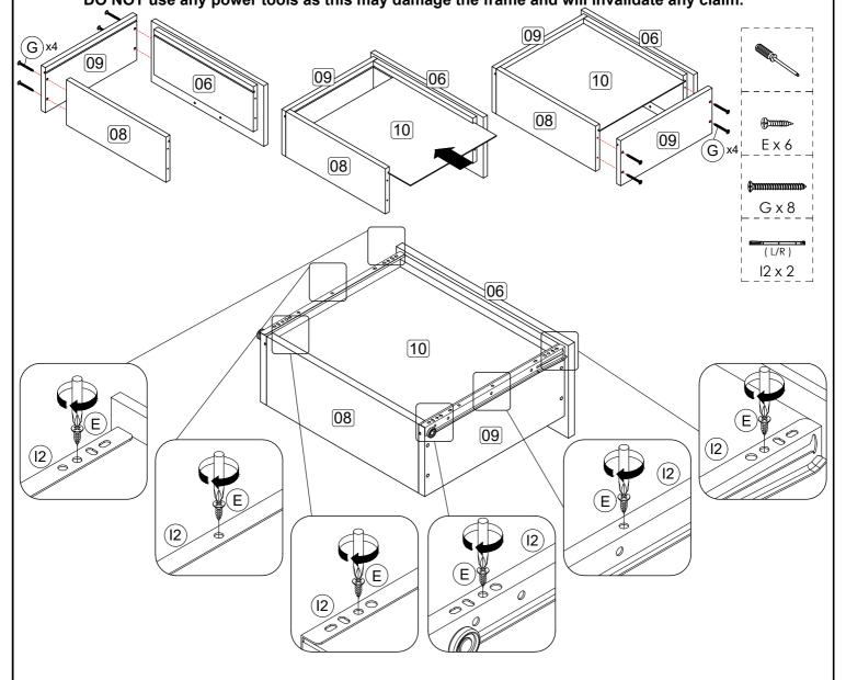
Step 7: Assemble the drawer components using hardware E, G and I2.
