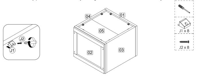
Step 6: Assemble the drawer components using hardware E, G and I2.
