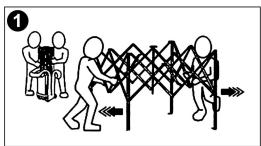
.After taking everything out of the carry bag, Place the gazebo frame in the center of the area to be sheltered. Stand on opposite sides, grasp outer legs, lift off the ground and pull out, and be careful not to pinch fingers.
