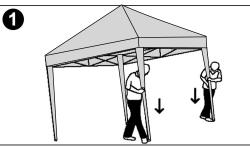
To make the tent stable, that must use reinforcement nails during installation. After the installation, you need to check whether the facility is fixed. If used regularly, the stable structure of the tent needs to be checked periodically.
