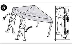
Lift each leg and slide the lower leg extension until the snap is locked.
