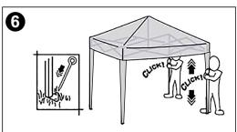
For height or leveling adjustment, depress leg latching buttons and slide the lower leg extensions as required to latch at any of the three adjustment holes. Put the four ground spikes through each hole in the bottom legs to secure them to the ground.
