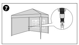
Two velcro stickers need to be fixedhere. The first piece needs to be passed under the hook, asshown in the picture, and the second piece needs to begiven in the middle of the elastic rope, as shown in the Picture, because it can help. Your tent is better protected against strong winds.
