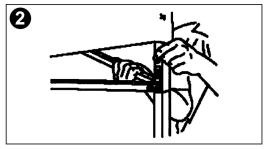
Release the auto slider at each top corner by pushing the snap button, and repeat at all four corners.
