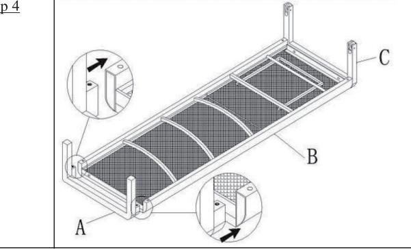
Insert the Front Leg(A) into the Seat Panel(B)
