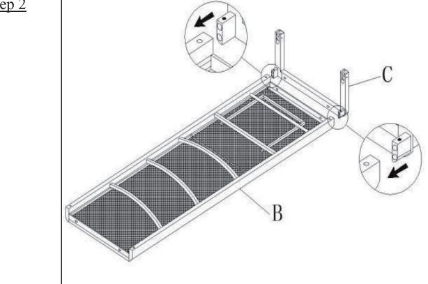
Insert the Rear Leg(C) into the Seat Panel(B)
