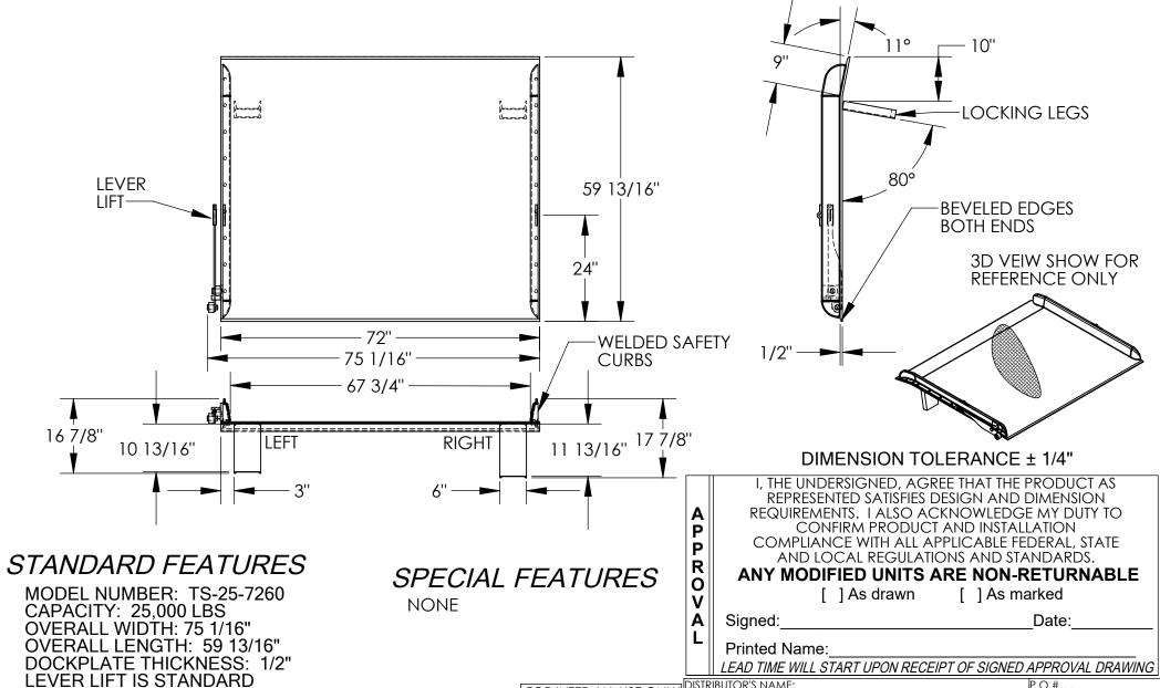
DISTRIBUTOR'S NAME: FOR INTERNAL USE ONLY PROJECT SIGN OFF LOCKING LEGS ARE 6" WIDE VESTIL MANUFACTURING RIGHT LEG LENGTH IS 11 13/16" **SALES** LEFT LEG LENGTH IS 10 13/16" ADL 12/21/2005 CROWN IS 11° & 9" FROM EDGE ENG. REFERENCE: X **HEIGHT DIFFERENCE: 10"** FAB. **DURABLE LIQUID PAINT BLUE FINISH** QUOTED LEAD TIME: X QUOTE # POWER Χ
