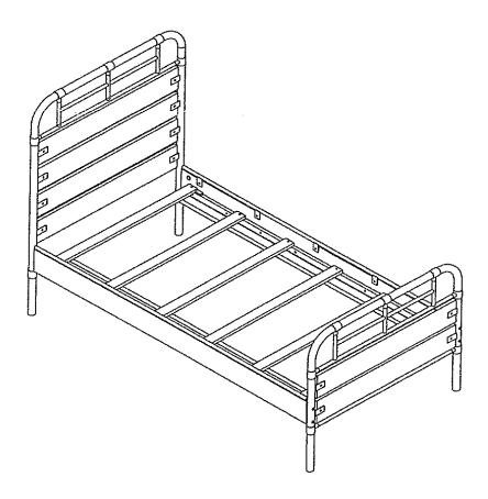
IMPORTANT: Do not tighten bolts completely until all bolts are completely lined up and inserted into holes
