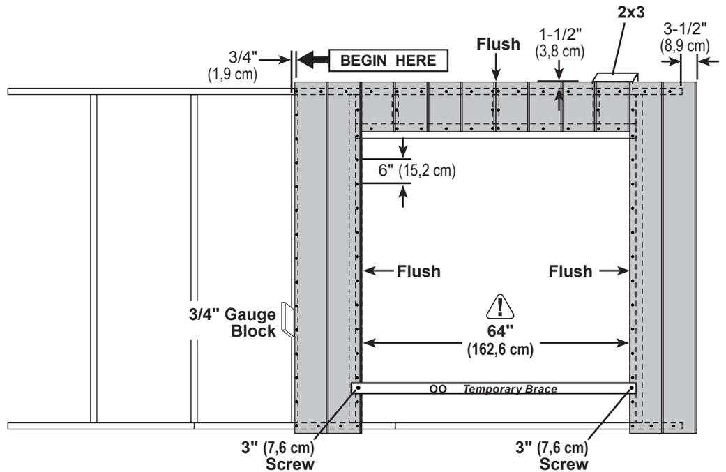
Secure panel with 2" nails spaced 6" apart on edges.
