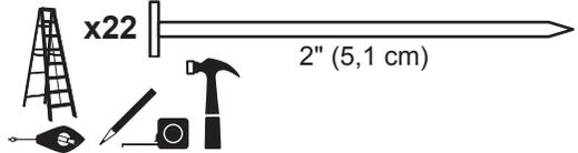
**3** Install 23-7/8" x 48" roof panel flush to the installed panel and flush at the peak (**Fig. B**). Secure panel with (1) 2" nail in each corner (*see: Fig. A*).
