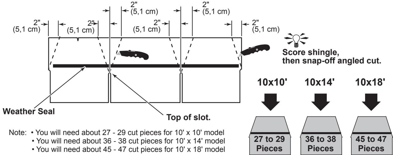
**2** Install first ridge cap flush to shingles at front, as shown.
