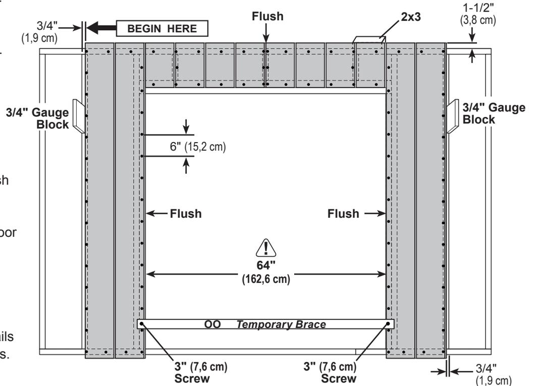
**5** Install (2) 11-7/8" x 84" panels flush to installed panels and 1-1/2" from the top plate.
