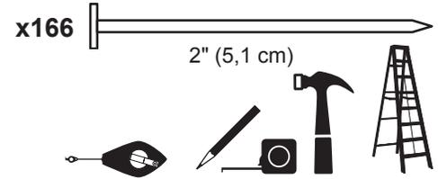
**8** Secure all roof panels with 2" nails spaced 6" apart and 12" apart inside of the upper panels.
