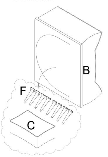
Step 2: Assemble back to seat using large bolts, spring washer and flat washer. Do not fully tighten any single bolt until all of them are align to the holes then fully tighten them by the short side of wrench.
