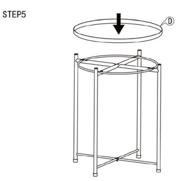
If the tray is unstable, adjust the screws in the STEP4 with a wrench to stabilize it
