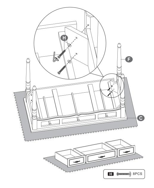
Semi-tighten the screws and fully tighten them after step5.
