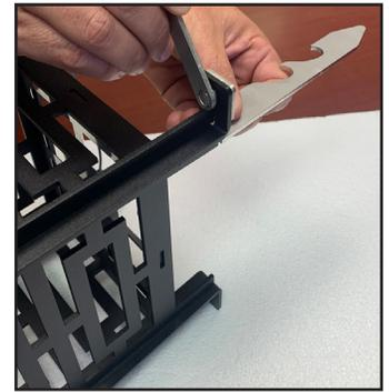
Use wrench provided to tighten locking screw.
