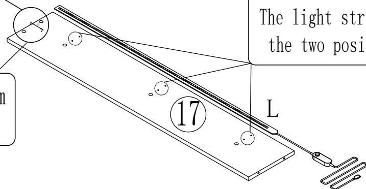
The light strip is pasted between the two positioning holes
