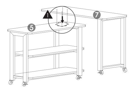
Position the upper table so that the holes in the lower table align with the screws on the bottom of the upper table. This will allow you to use a screwdriver by inserting it through the holes in the lower table, so that you are able to tighten the screws on the bottom of the upper table.
