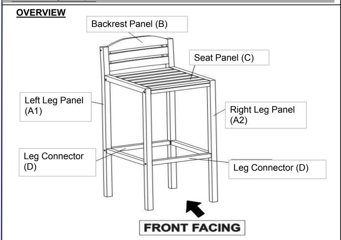
This Bar Stool has multiple parts and may require up to 30 minutes to assemble. To give you an overview of the Bar Stool parts, the above picture is to help you put the various parts into perspective. Please read through the instructions below to familiarise youself with the parts and steps before assembly.
