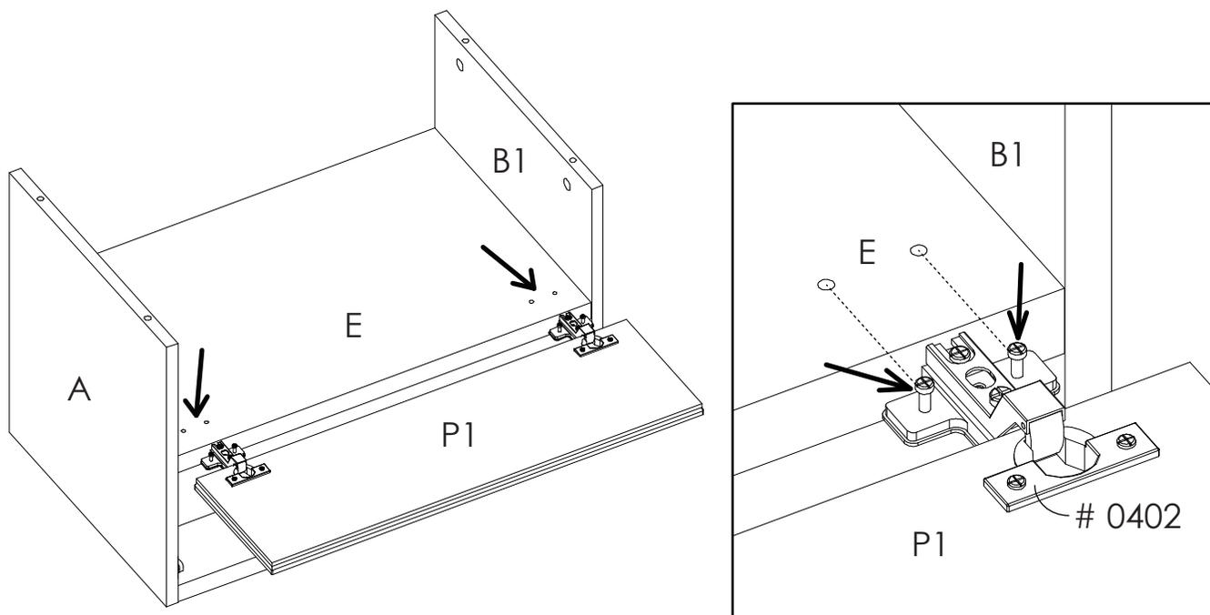
**8** Fasten the panel C to the assembled unit. Then, tighten the 4 cam locks # 0203 located on panels A and B1. Add 1 cap # 2194 on each cam lock
