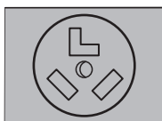
3-Wire Receptacle (NEMA Type 10-30R)
