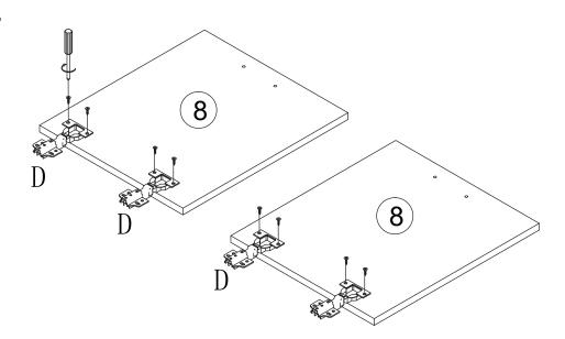
First, install a pair of D on 8, and install another door panel in the same way.
