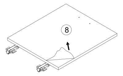
After installing D, tear off the coating on the front of 8.
