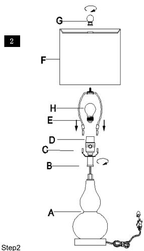
Insert the Harp (E) into the Saddle (C).
