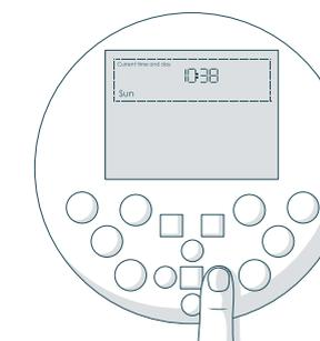
2. Use the LEFT and RIGHT buttons to move between minutes, hours, and days of the week. Use the FWD and BACK buttons to adjust your selection.
