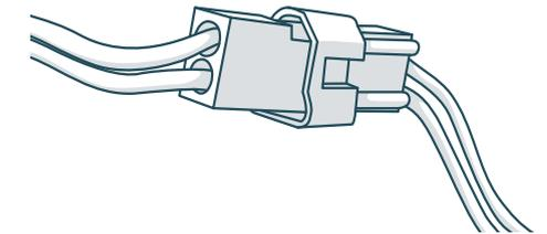
2. Disconnect the old battery by pulling the plug, not the wires. Plug in your new battery.
