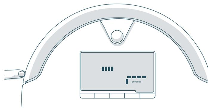
Press the left side of Bob’s bumper, and the bar to the left of the word “checkup” should light up; press the right side of the bumper, and the bar to the right of the word “checkup” should light up. Press the center of the bumper, and both bars on either side of the word “checkup” should light up at the same time.
