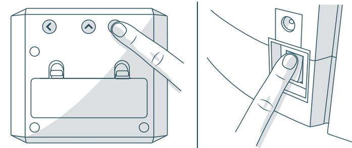
3. Hold down the SYNC button while at the same time flipping Bob's power switch ON.
