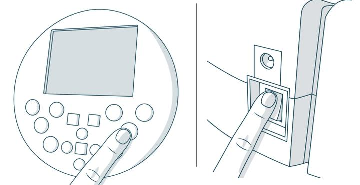
2. While still holding down the OK/SYNC button, flip Bob's power switch ON.
