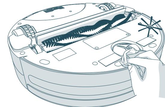
1. Wipe the obstacle/wall and edge sensors with a soft cloth slightly dampened with cold water or alcohol.
