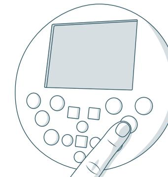
2. While still holding down the OK/SYNC button, flip Bob's power switch ON.
