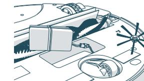
Unplug the battery, wait 30 seconds, and then reconnect the battery.
