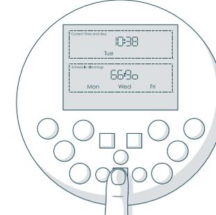
2. Press the STOP button and “bbgo” (back-to-back go) will appear on the remote’s screen.
