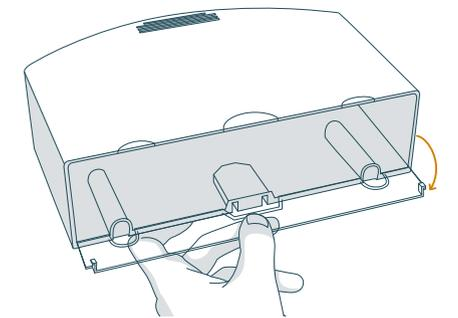
2. Carefully open the plastic gate and dump out the contents of the dustbin.
