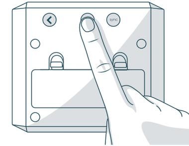
1. Press the
