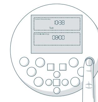
1. Press the SET CLEANING SCHEDULE button on the remote. The first hour digit will start flashing.
