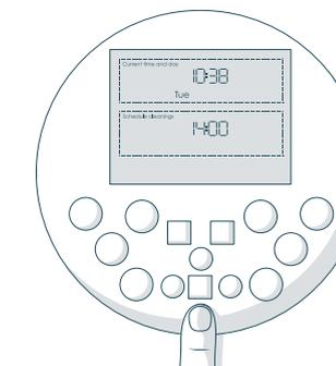
2. Use the LEFT and RIGHT buttons to move between minutes, hours, and days of the week. Use the FWD and BACK buttons to adjust your selection.
