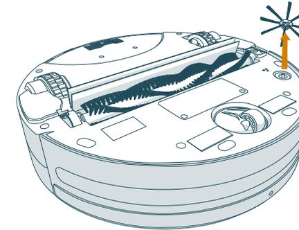
1. Remove the screw on the side brush using a flat head screwdriver.
