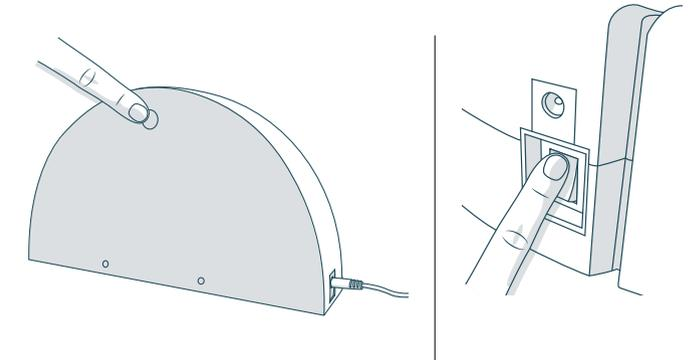
2. Hold down the SYNC button on the back of the charging station while at the same time flipping Bob's power switch ON.
