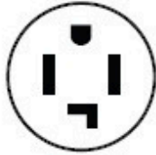
4-Wire receptacle (14-30R)
