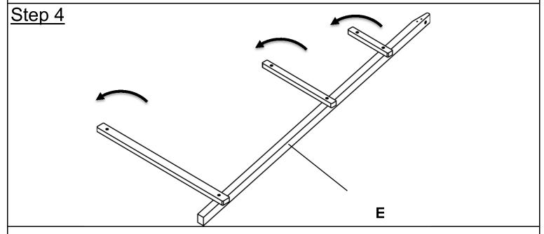
Rotate the Leg Support Bars of First Legs(E) 90 degrees as pictured above.
