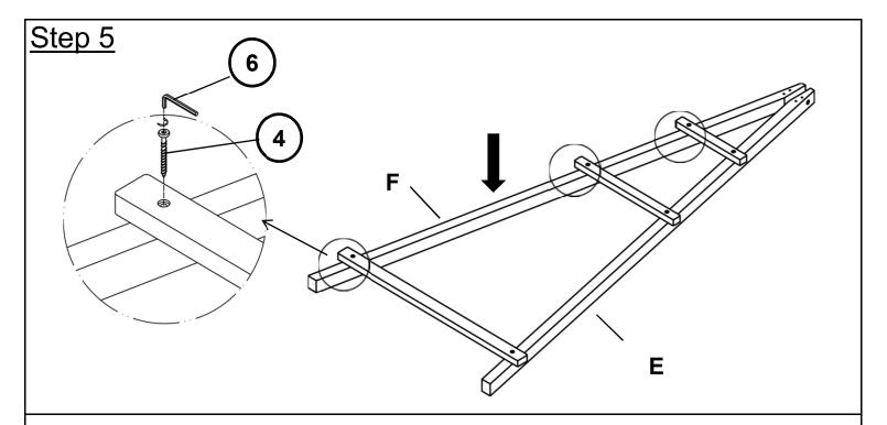
Attach Second Legs(F) to the Leg Support Bars of First Legs(E) using Screws(4) with Allen Key(6) as pictured above.
