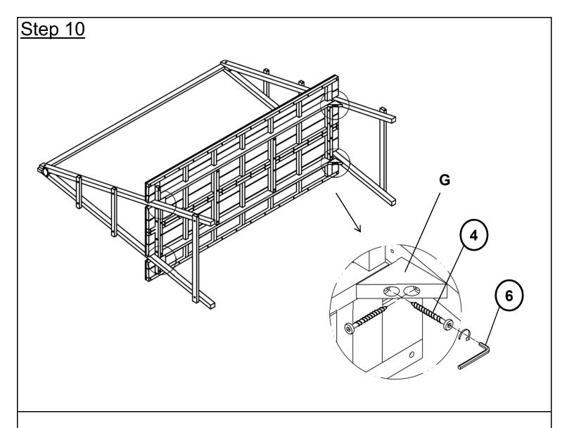
Attach Corner Blocks(G) to Leg Frames and Table Top using Screws(4) with Allen Key(6) as pictured above.
