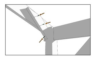
Place an end brace against the inner face of the outer runner so that the lower face is butted against the inner face of the post and the top edge is approximately 10mm from the top edge of the rafter. Fix in place with 2 x 65mm screws into the rafter and 1 x 75mm screw into the post as shown. Repeat for the other end of the structure.
