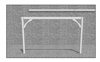
Using your assistants, manoeuvre the previously assembled "goalpost" with 2 posts into place. Position it parallel to the wall with the runner overhang adjacent to the outer end of your wall plates. Consult the Panel length table (page 3) to correctly distance the posts from the wall.
