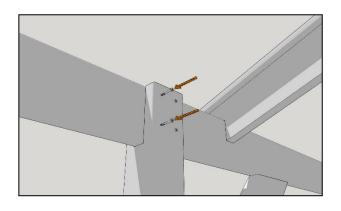
... before securing it into place with 2 x 65mm screws through the post into the runner.
