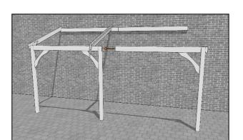
Using your assistants again, manoeuvre the previously assembled "goal post" with 1 post into place. Slide the free runner end into the slot in the centre post pushing it fully home until it butts against the other runner...
