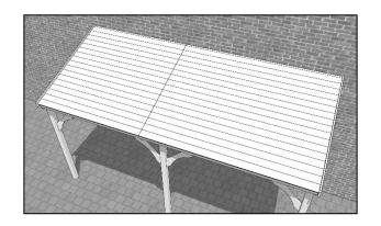
Slot the fascia panel into place so that it is butted up against the underside of the roof and against the rafter ends before fixing in place into the outer rafter at both ends with 2 x 45mm screws ...
