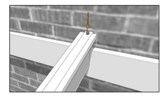
Now fix the intermediate rafter into place with a 120mm coachscrew driven down into the wall plate...
