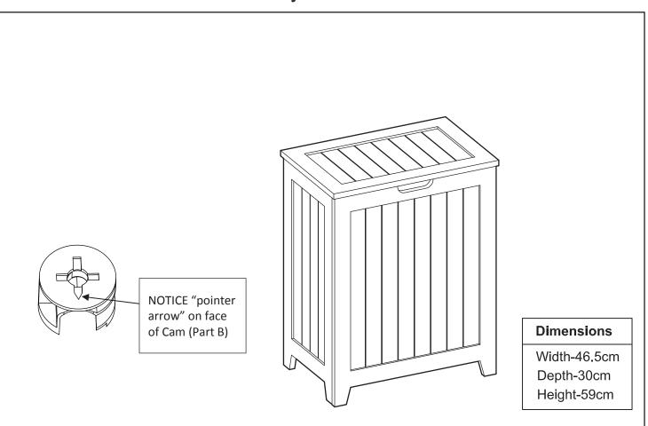
Place the Cam so that the "pointer arrow" faces the edge of the panel. This allows for the Pin (Part A) to be correctly aligned with the opening of the Cam.
