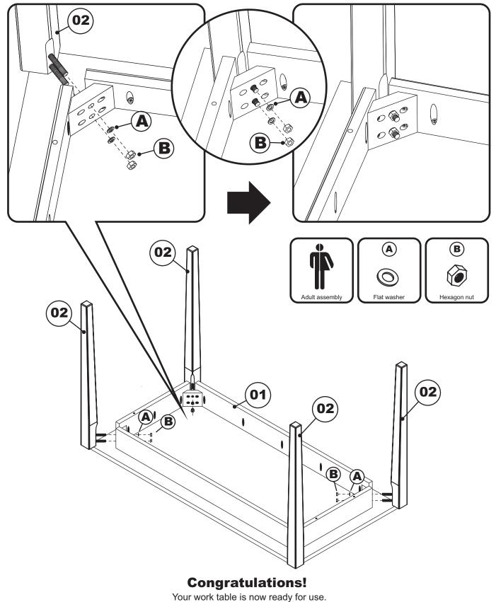
We recommend that you recheck that all screws are tight, and that all parts are secure before use and periodically to ensure lasting safety.
