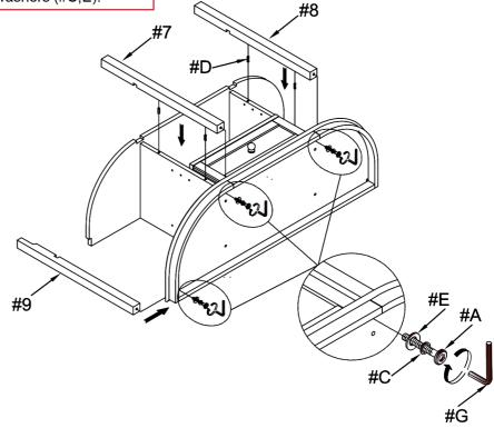
Align top (#10) to the unit, then secure by using bolts (#B) with washers (#C,E).
