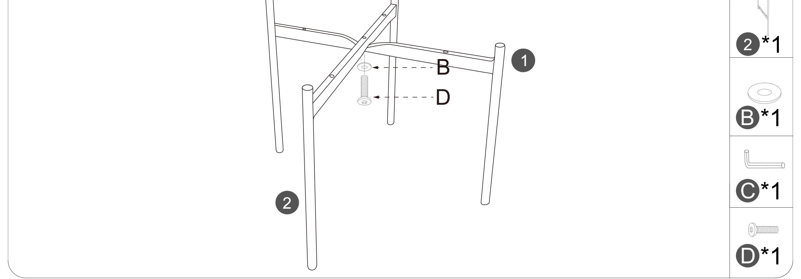
Attach legs to the backside of seat cushion(3) using washers(B) and bolts(A). Do NOT fully tighten the bolts until all of them are
