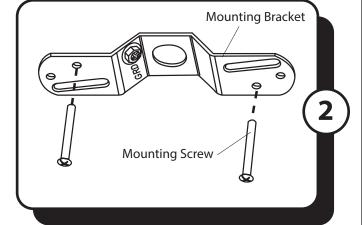
2. Insert the mounting screws into the holes in the mounting bracket as shown.
