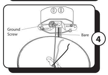
4. Loosen the ground screw on the mounting bracket and wrap the bare wire from the fixture around the ground screw. Tighten the ground screw to hold the bare wire in place. **Note:** Ensure there is enough of the bare wire extending from the ground screw to connect to the ground wire from the outlet box using a wire connector.
