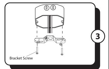
3. Use the bracket screws from the hardware bag to attach the mounting bracket securely to the outlet box.
