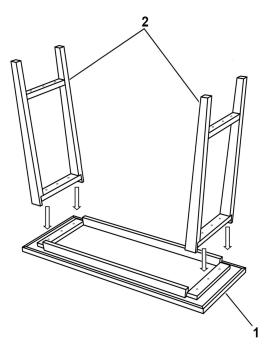
STEP# 2: Tighten the bolts to lock the legs as shown below.
