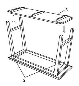
STEP# 4: Tighten the bolts to lock the Shelf as shown below.
