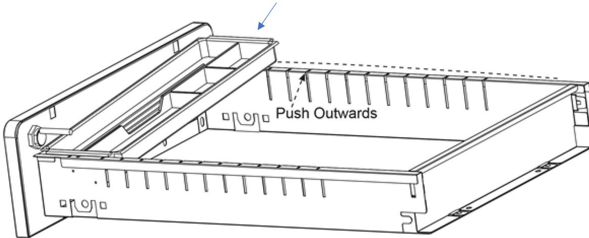
Install or adjust the file bar, make sure the bar is in its correct direction
