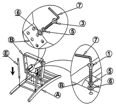
**Step 2:** Attach front legs (D) to the seat frame (B) with bolts (2), washers (5) and (6). Tighten with allen key (7).
