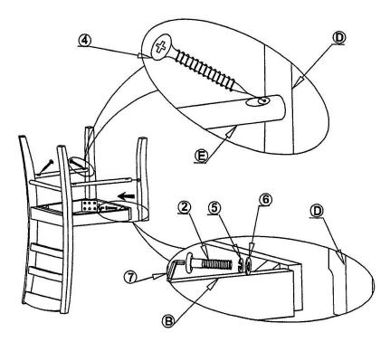
**Step 3:** Attach seat (from step 2) by using screws (4), tighten with screw driver.
