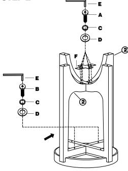
NOTE: DO NOT TIGHTEN ALL THE BOLTS UNTIL THEY ARE INSTALLED IN CORRESPONDING HOLES!
