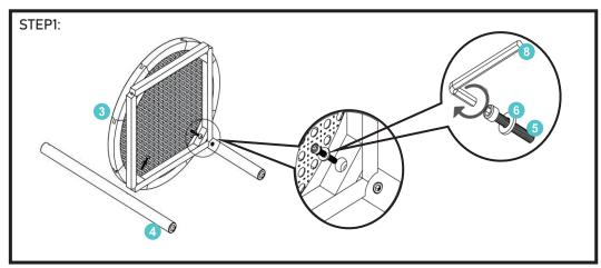
Step 1: Put the **(3)** on the **(5)**, pass through the corner hole of the square frame on the bottom of the shelf, screw it into the holeon **(4)**.
