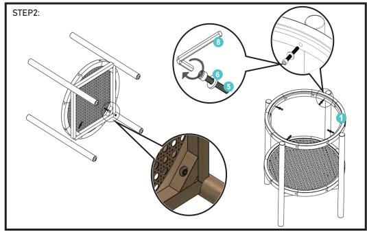
Step 2: In the same way, lock the other two legs, as shown in effect picture . Straighten the support feet, connect the panels, and tighten them with ③.
