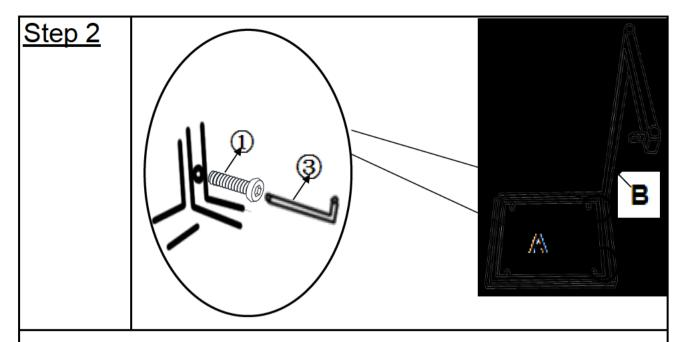
Attach the Side Panel(B) to Top Panel(A) using Bolts(1) with Allen Key(3) as shown above.
