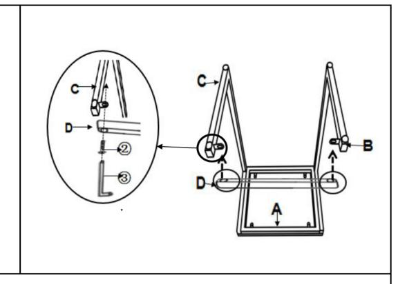
Attach the Base Support Bar(C) to Side Panel(B) and Side Panel(C) using Bolts(2) with Allen Key(3).
