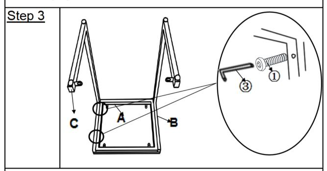
Attach the Side Panel(C) to Top Panel(A) using Bolts(1) with Allen Key(3) as shown above.
