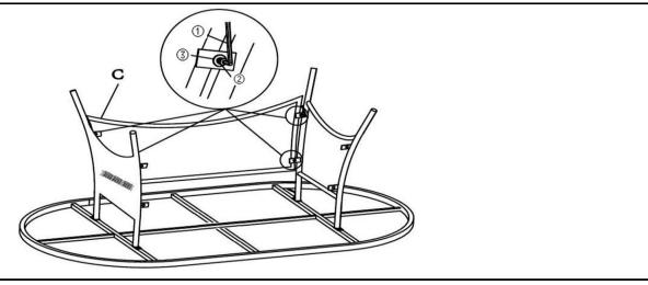
Attach Leg Support Panel(C) between Leg Panels(B) using Bolt(2) and Washer(3) with Allen Key(1) as shown in the picture above.
