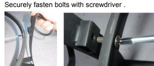
2. According to the same method above , assemble all stand legs but bolts cannot be twisted too tight .
