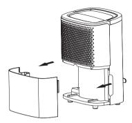
NOTE: Do not remove the float from the water tank. The water full sensor will no longer be able to detect the water level correctly without the float and water may leak from the water tank.
