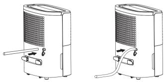
CAUTION: DO NOT PLACE CONTINUOUS DRAINAGE HOSE OUTSIDE IN TEMPERATURES BELOW 1°C
