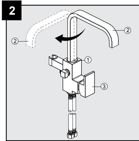
Loosen the set screw (1) pre-assembled to the spout (2), rotate the spout (2) about 90° to align handle (3), then tighten the screw.
