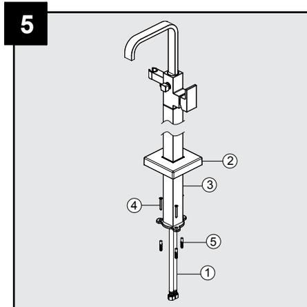
Place the assembly with the flexible supply lines (1) through the prepared hole and then holding the escutcheon (2), secure the standpipe (3). Note: If mounting into wooden floor, secure the standpipe (3) using screws (4) only (wall plugs are not needed). If mounting into solid floor, mark the position of holes first and then secure the standpipe (3) using anchors (5) and screws (4). Where required ensure correct anchors for your floor type are used.
