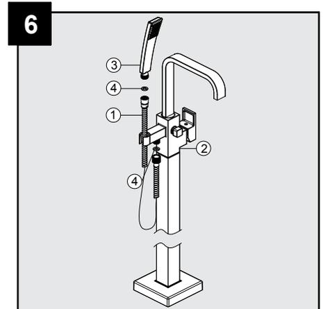
Connect one end of the shower hose (1) to the mixer (2) and the other end to the hand shower (3). Ensure the washer (4) is in each end for seal.
