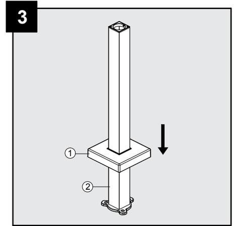
Place the escutcheon (1) over the standpipe (2) and then push it to the base.
