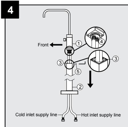
Attach the mixer (1) to the standpipe (2), make sure the prongs (3) on the standpipe (2) insert into the hole (4) of the mixer (1). Install the set screw (5) and tighten into the standpipe (2) with hex wrench. Note: Do not to reverse the cold and hot supply lines.
